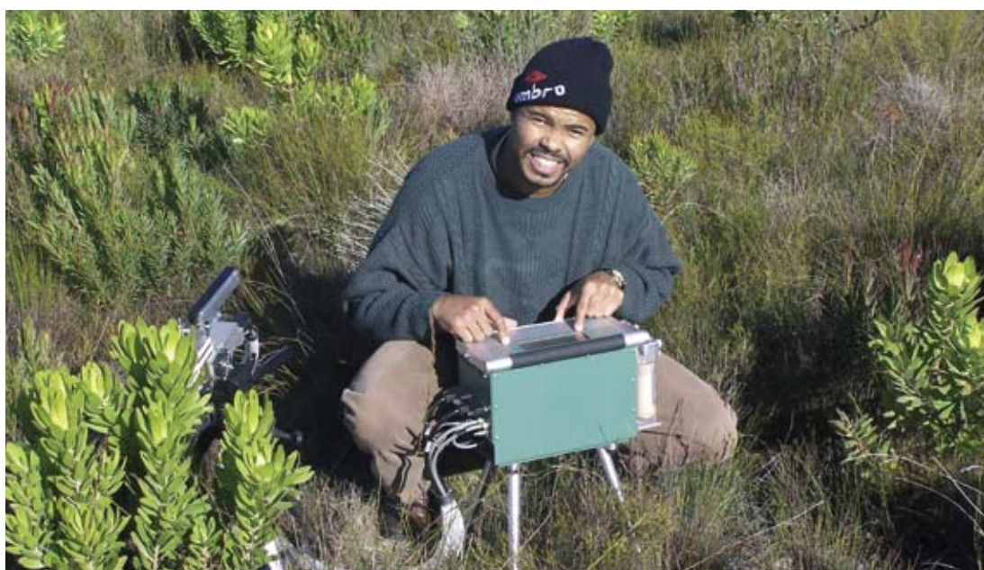
Barney Kgope uses an infra-red gas analyser to measure photosynthesis of proteas at Silvermine.
