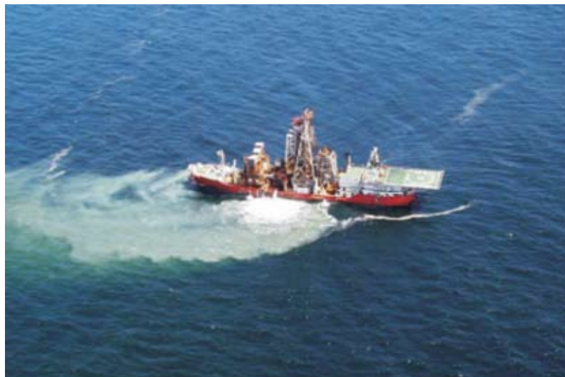
FIGURE 2.3.—Coarse sediment discharge plume during mining operations (Penny 2005).
