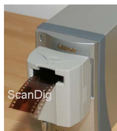
Scanning a 35mm film strip with the serial SA-21
