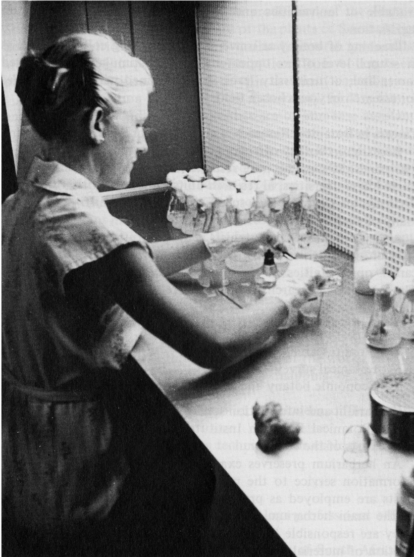
Figure 3. Preparation of material for tissue culture must be undertaken in the absolutely clean environment of a laminar-flow bench.
